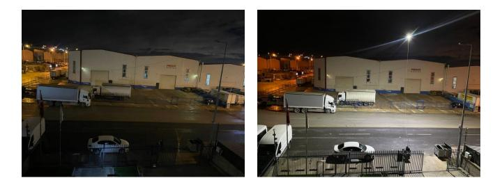
In the illumination test performed by taking our wired illuminated aircraft to an altitude of 10m (AGL), 147lux was obtained on the ground, 68 lux at an altitude of 15m (AGL) and 41lux was obtained in the illumination measurement made while flying at an altitude of 20m (AGL). The visuals of the results of the measurements made with the Luxmeter at 10m, 15m and 20m are as follows.
